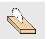
• For handling and cutting of STEICO LVL, as with softwood, please use standard wood working tools and machinery along with the appropriate PPE (Personal Protective Equipment).
